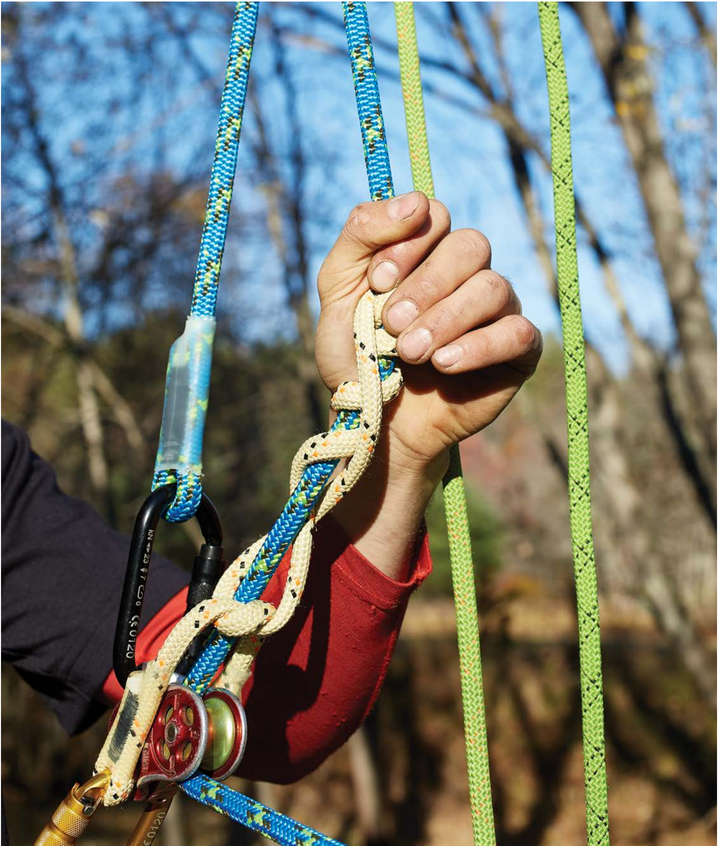
9 mm RIT Eye-and-Eye used in conjunction with the Scion™ Climbing Line. HTP™ Bicolor used as access line.
