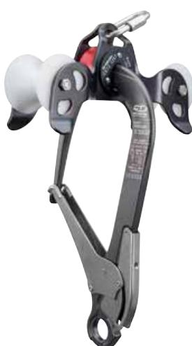
Combined anchor and pulley for evacuation from cable cars and chair lifts. It allows evacuation by allowing rescuers to be lowered along the cable, or when the underlying terrain permits it, to allow the unloaded pulley to run down the cable to the desired position and then use it as a winch and lower anchor.
