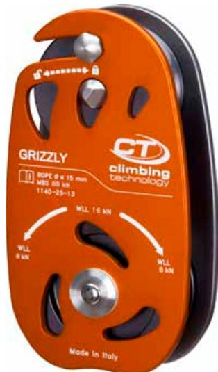
Pulley for tree felling for high loads 80 kN, with aluminium pulleys mounted on self-lubricating bushings with steel pivots and aluminium flanges. Very simple and safe opening system: pressure on the upper pivot allows a 90° rotation of the front flange.
